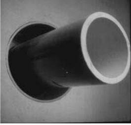
1. Center the pipe, cable or conduit in wall opening or casing. Make sure the pipe will be adequately supported on both ends. Link-Seal® modular seals are not intended to support the weight of the pipe.
