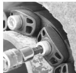
5. **LS-200 thru. LS-315** Using a hand socket allen head or off-set wrench **ONLY**, start at 12 O' Clock. Do not tighten any bolt more than 4 turns at a time. Continue in a clockwise manner until links have been uniformly compressed. (Approx. 2 or 3 rotations)
