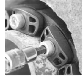
5. **LS-200 thru. LS-315** Using a hand socket allen head or off-set wrench **ONLY**, start at 12 O' Clock. Do not tighten any bolt more than 4 turns at a time. Continue in a clockwise manner until links have been uniformly compressed. (Approx. 2 or 3 rotations)
