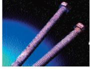
1,470 hour salt spray test performed by an independent laboratory. Test results are available on request.
