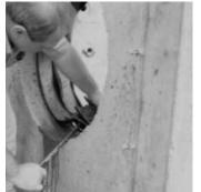
**10.** Remove disks by breaking out the entire assembly.
