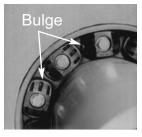
6. Make 2 or 3 more passes at 4 turns per bolt MAX-IMUM, tightening all bolts clockwise until all sealing elements "bulge" around all pressure plates. On type 316 stainless steel bolts, hand tighten ONLY without power tool.
